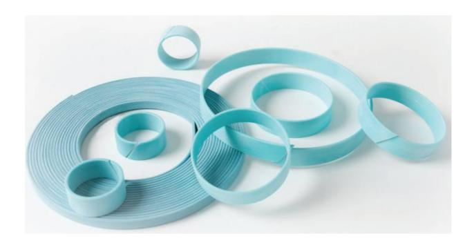
GTN is intended for use as wear strip within hydraulic cylinders. It is supplied in 10 metre length coils although longer lengths are available on request and is supplied with chamfered edges. The material is a high load composite bearing material made from synthetic fabric reinforcement, which is impregnated with a thermosetting resin system. The material is pigmented Turquoise (blue/green colour) to suit specific customer requirements.
